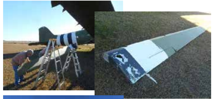
Above, a damaged aileron that will be reskinned in aluminum as the rest of the control surfaces Below, Arvid Pomeroy and Dave Smith work at making the interior accessible.
