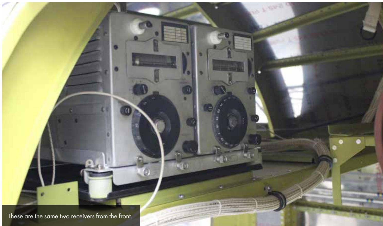
The vented backsides of the two SCR 274 receivers (grey) show in this angle. These are the newly overhauled units from John Castorina.
