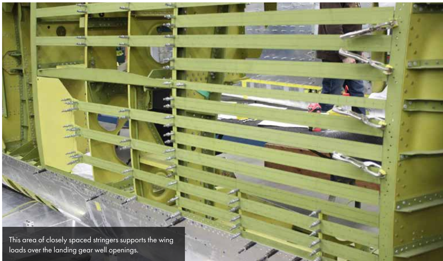
The engineering drawings identify these smaller spanwise elements as “stringers” despite that name being more commonly used for fuselage components.
