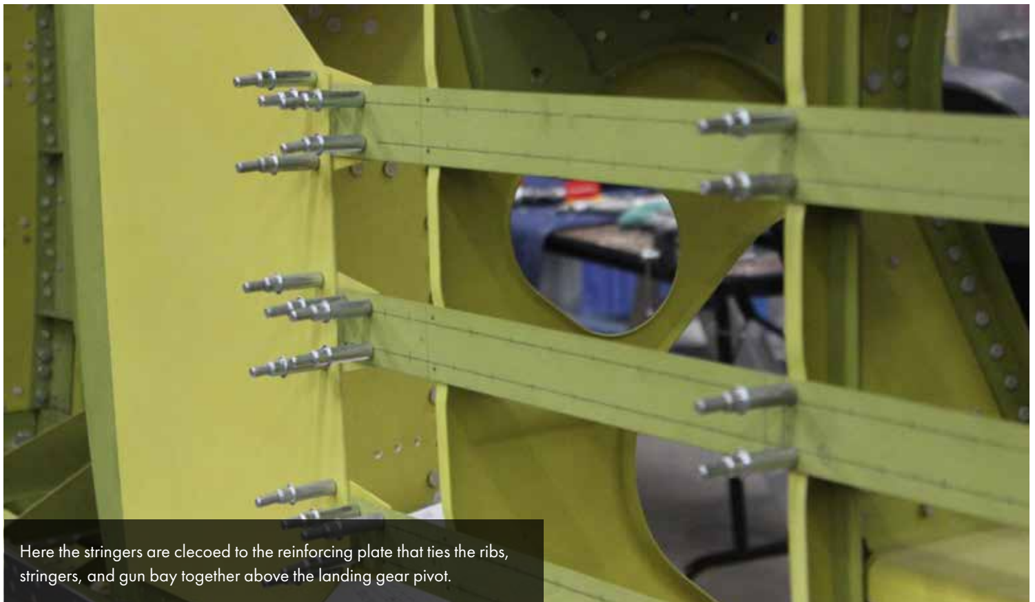
This image gives perspective on the placement of the stringers detailed in the previous photos.
