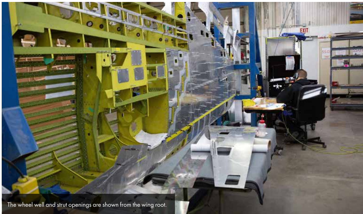
This angle shows the wheel well and the openings that allow the main gear strut to retract into the wing, looking from the wing tip end.
