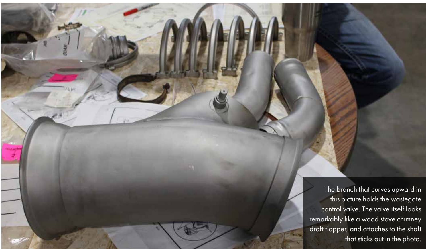
These are parts for the main exhaust assembly, the exhaust ring around the cylinders of the R-2800. All will be inspected, and some will be found restorable to service.
