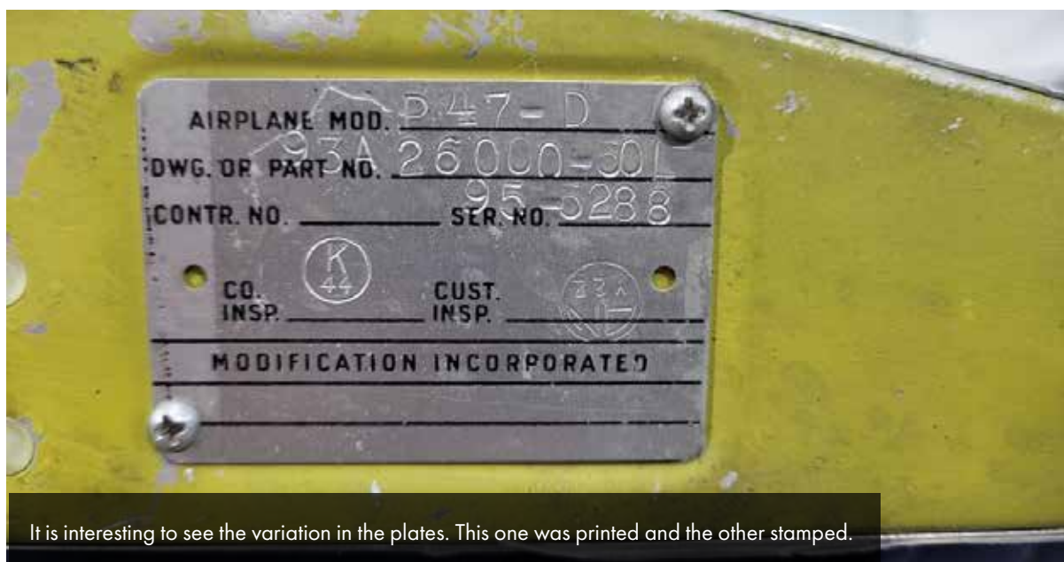
These assembly data plates are original and will be used in the restoration.
