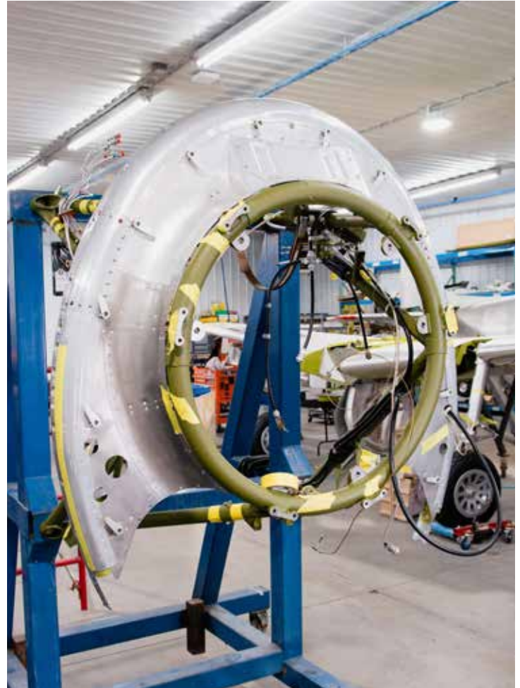
Aaron is assembling the Quick Engine Change assembly (QEC) for the P-47 in anticipation of the overhauled R-2800's arrival.
