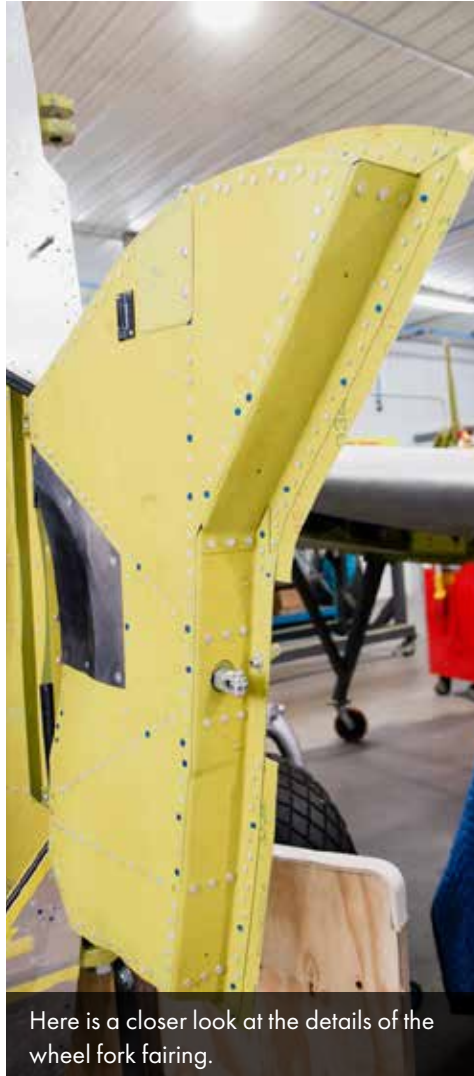
The door lock mechanism protrudes from the wheel fork fairing.
