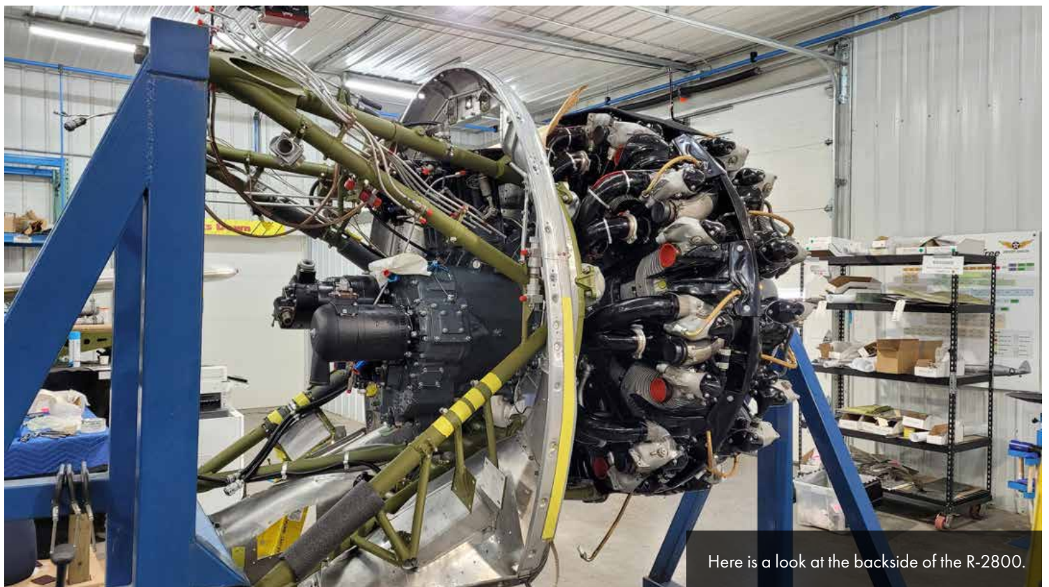
A huge milestone was reached this month when the overhauled R-2800 came in from Anderson Aeromotive of Grangeville, Idaho! Before installation on the P-47, the engine is mounted in this jig to ensure a perfect fit to the engine mount.
