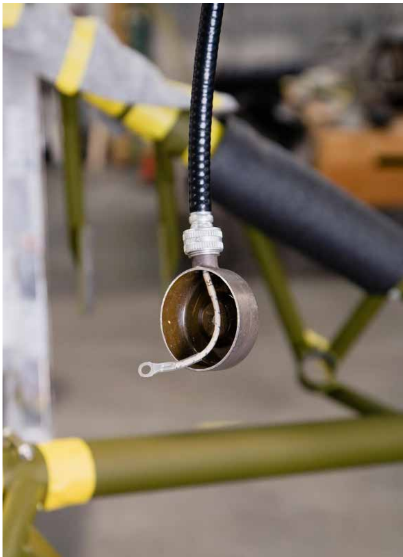
This electrical harness and cap connect to the oil dilution solenoid. Oil was slightly diluted with gasoline from the fuel tanks for cold weather starts.
