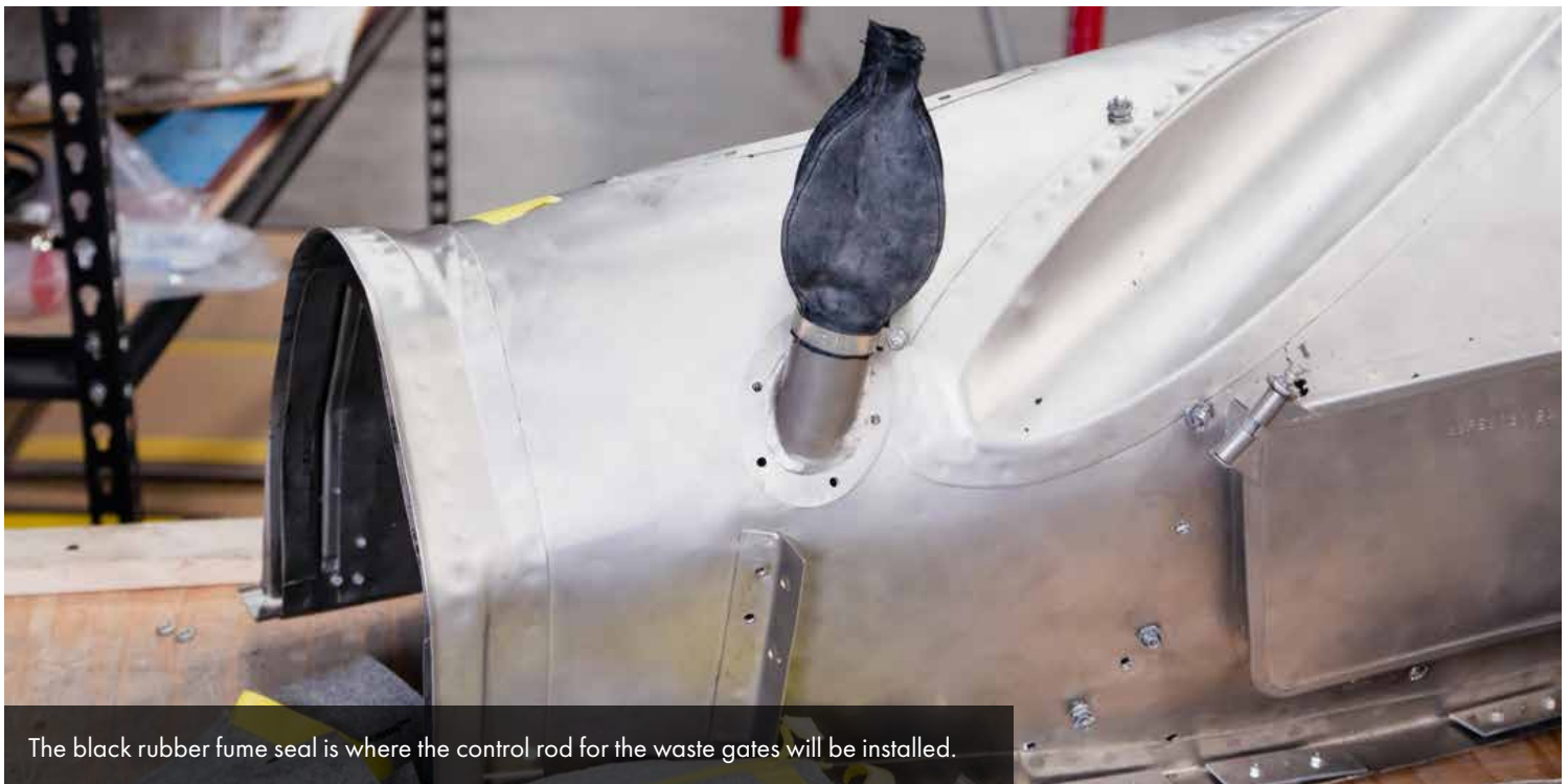
Forward shroud assemblies for each side sit on the workbench. Their function is to direct air to the oil coolers and past the waste gates.
