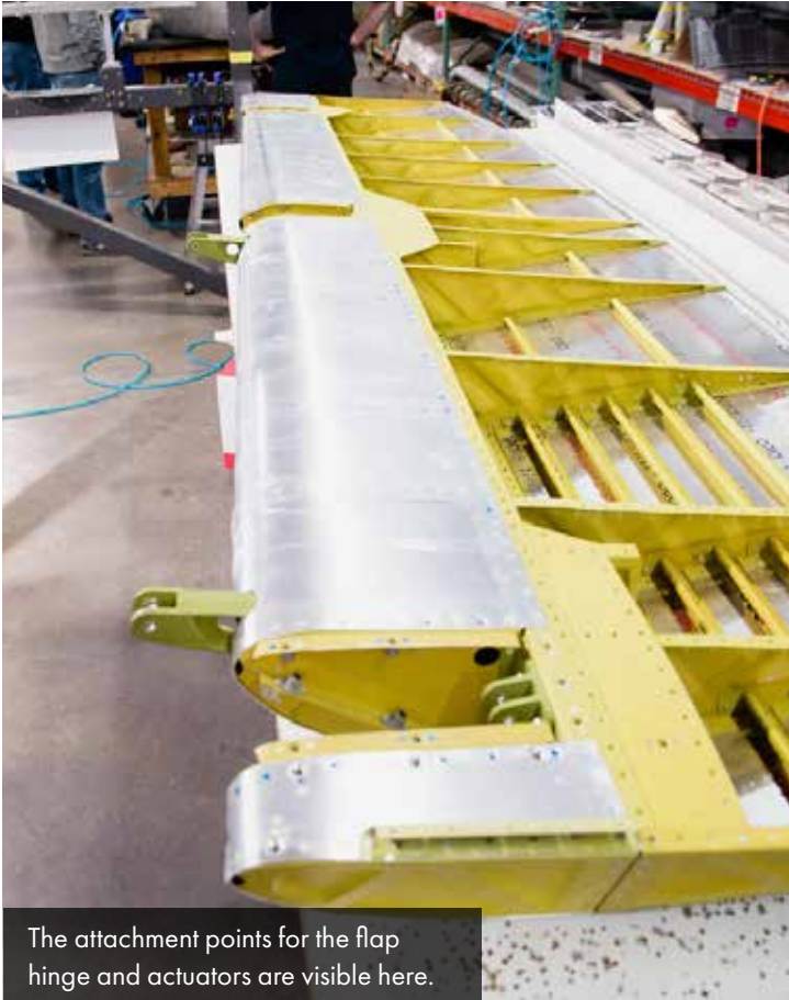
The control surface leading edges have a complex joint edge.
