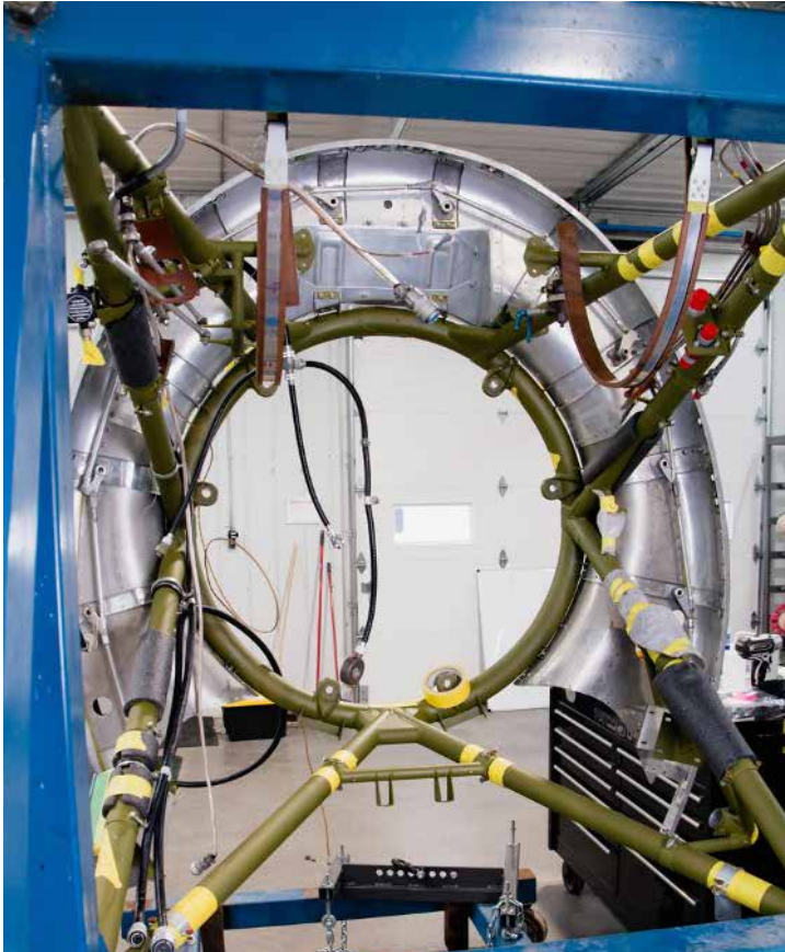
This is a view of the engine mount from behind. Near the cross brace in the lower center are strips of masking tape that demarcate the area that Aaron had to remove paint from. Paint removal was necessary because the ground clamps must attach to bare metal for a good electrical ground connection.
