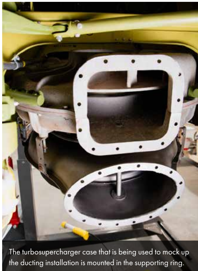
The turbine side of the turbosupercharger is on top in this image.
