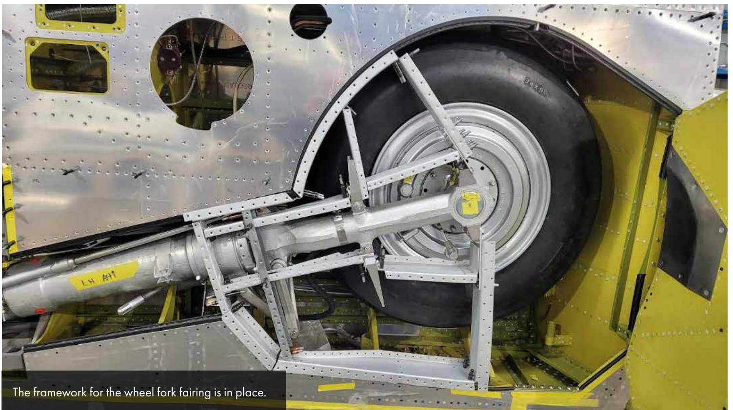
This image shows the plates that attach to the hub that serve as mounting surfaces for the wheel fork fairing door.
