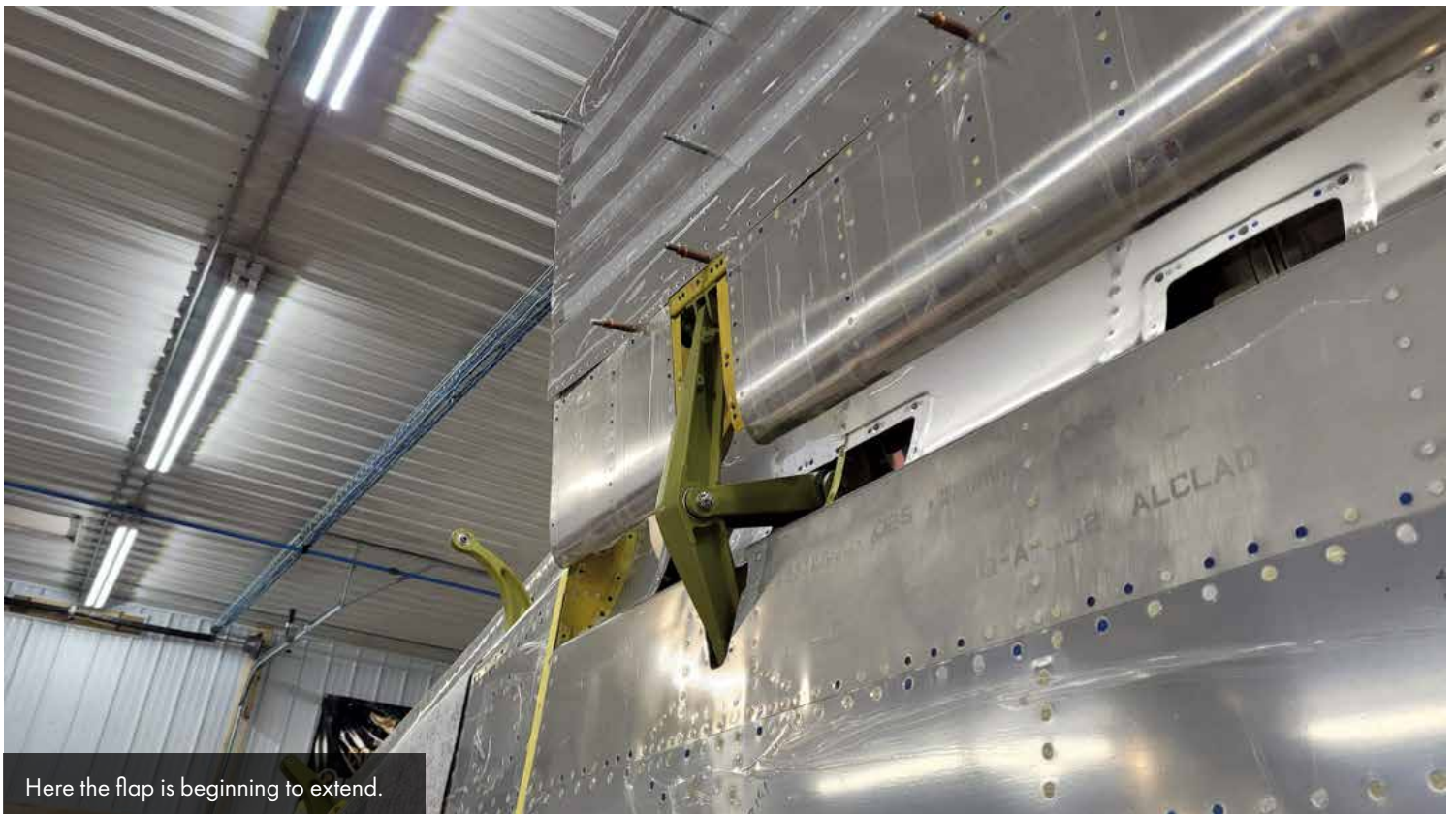
Mark uses a hydraulic test stand, sometimes called a mule, to test the operation of the flap.
