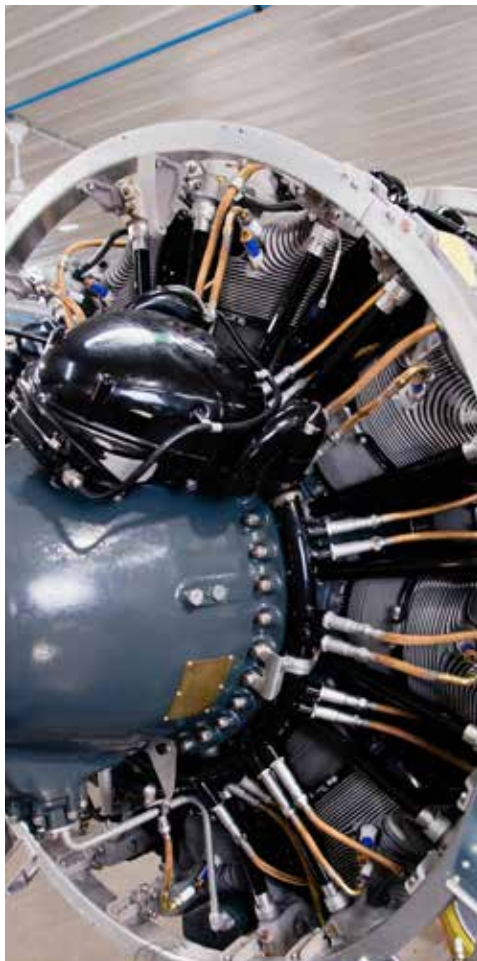
The bare aluminum cowl support rings are prominent in this photo. The cowl flaps are already attached to the rear ring.
