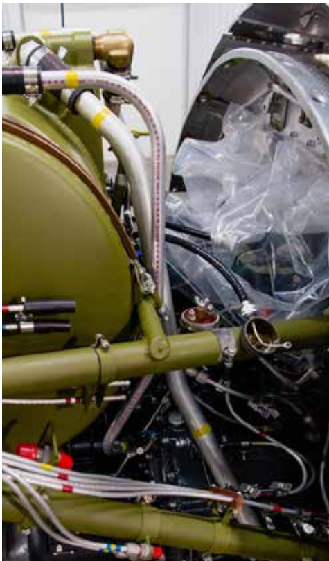
As the QEC assembly was done, many connections to engine accessories had to be made. Visible here are hydraulic lines with blue yellow blue tape coding, and the large uncoated metal oil line leading downward from the green painted oil tank in the center of the image
