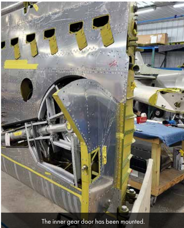
Here, the rivets have been driven and the same skin is permanently attached.
