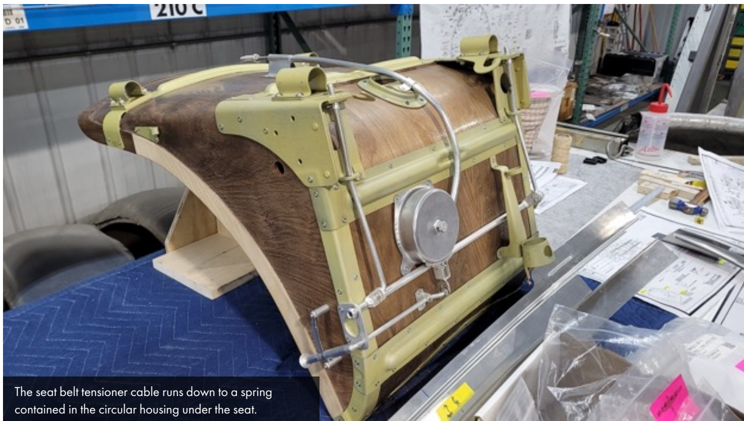
The metal parts of the seat have now been painted. The cable housing running up the back of the seat is for the seat belt tensioner.
