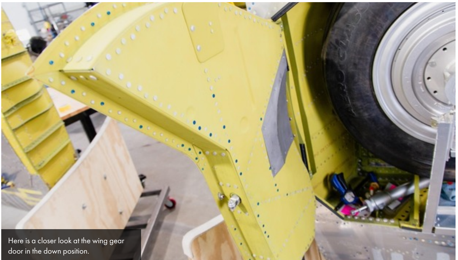
The inner main gear door (called the wing door by Republic) has been fitted.
