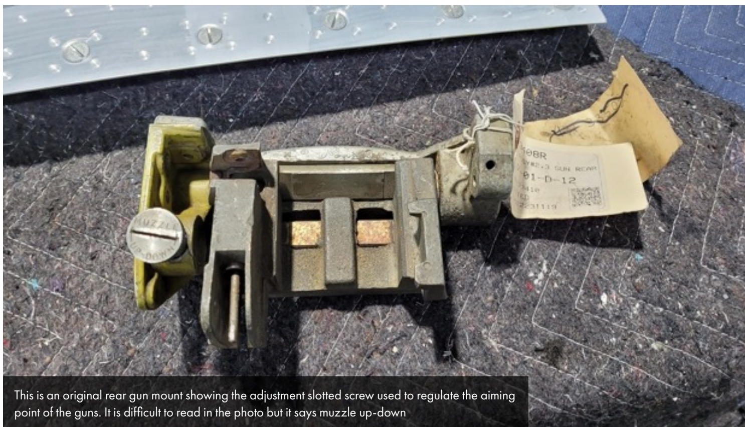
The rear gun mount levers work on a cam action to lock the rear of the M2 receivers in place.
