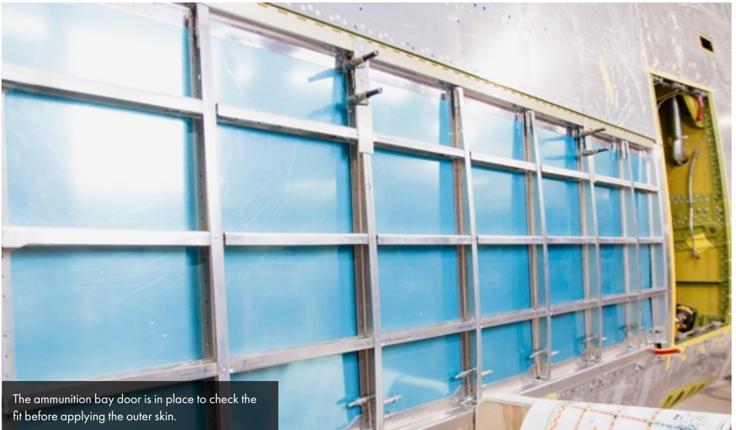
The gun bay cover door nears completion.
